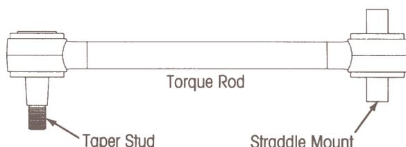
**Rubber Bushed Torque Rods:** The length of the torque rods is determined by the truck manufacturer for optimum drive line angles. The torque rods control these angles and also absorb driving and braking forces. The mounting brackets at the axle ends of the torque rods are furnished and welded into position on the axle housings by the axle manufacturer.
