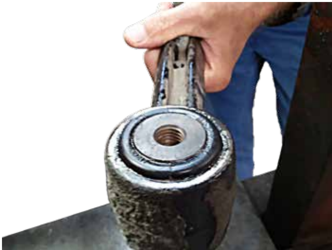
Check that the bush is centred in the torque rod end
