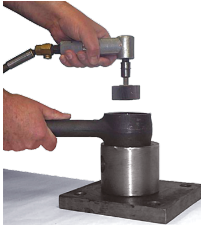
Clean rubber remnants out of torque rod ends
