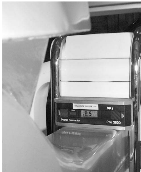
Figure 5 Measurement of Axle Angles (A4 + A5)
