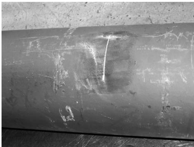
Figure 1. Previous bracket weld ground flush to axle tube surface
