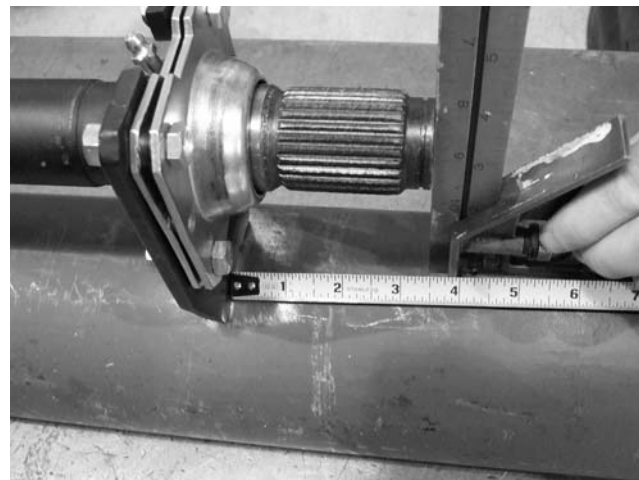
Figure 2. S-cam bracket assembly must be 3.5 inches (90mm) from the end of the camshaft
