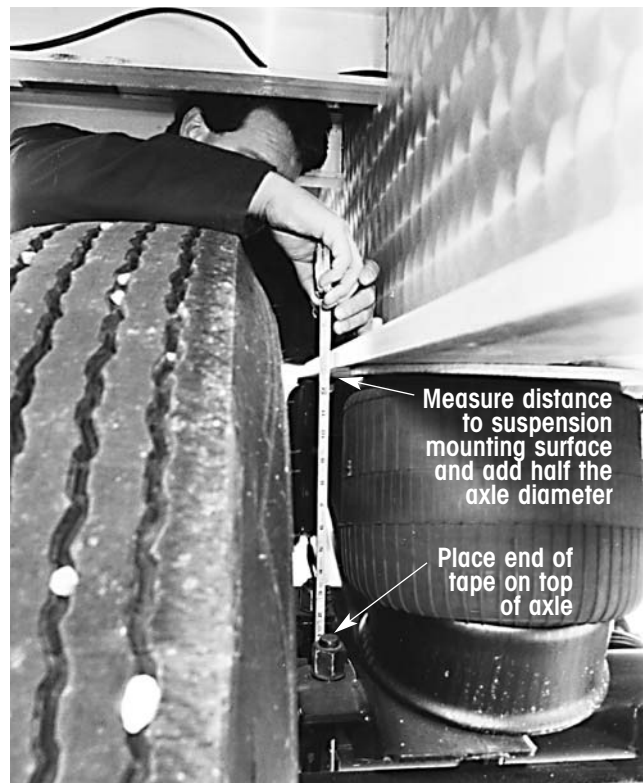
Figure 3. Measuring ride height
