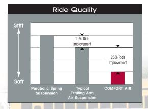
Using advanced spring technology from Hendrickson, COMFORT AIR's main support member has an elongated design for optimized roll stiffness. This provides a softer ride and greater protection from the effects of road shock on your chassis, equipment, drivers and passengers.
