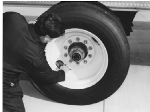
Figure 2: *Check air pressure in tires*
