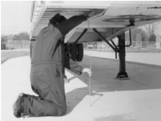
Figure 5: Measure from ground to kingpin
