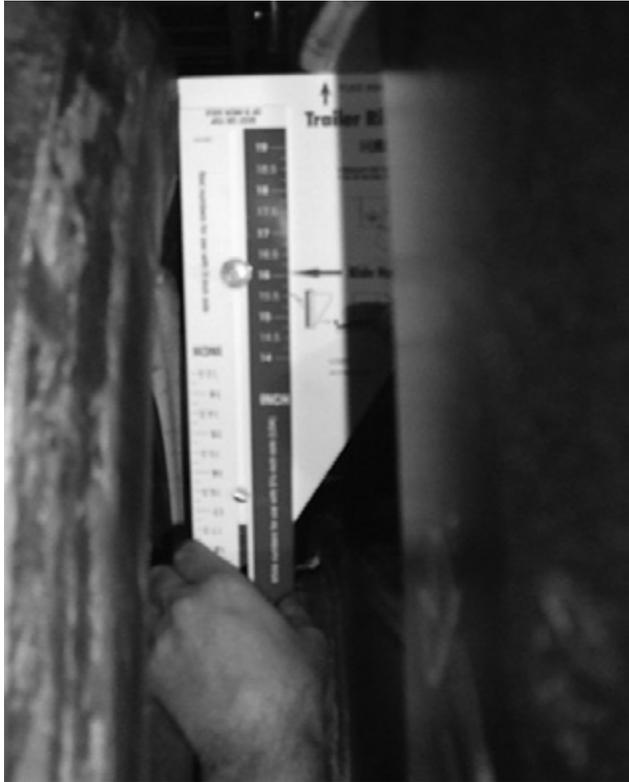
Figure 8: Using gauge to measure ride height
