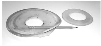
Examples of "worn-through" bushing tube spacers. The spacer on the right is an example of extreme wear. Its circumference has been completely trimmed by the bushing tube.
