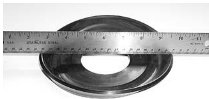
An example of a "cupped" bushing tube spacer. Friction-generated heat causes the spacer to "form" or "cup" around the bushing and bushing tube. This is normal as long as the bushing tube spacer remains intact and does not become cut or worn-through.
