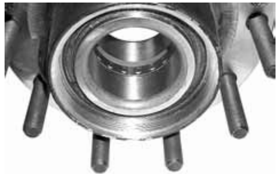
Figure 4: Normally present grease at hub outer bearing seal.
